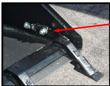
Pull Up Bolt Design Doing Its Job!
